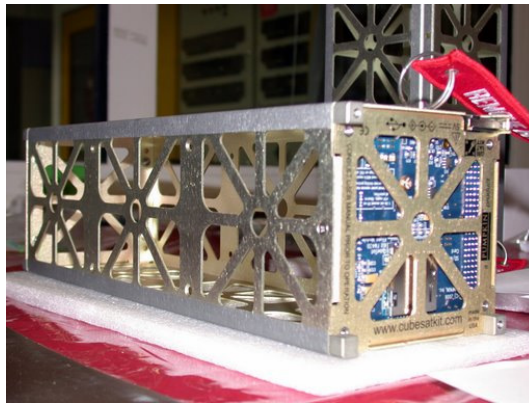
Figure 1- Rear cover with on board computer visible (FM430)
